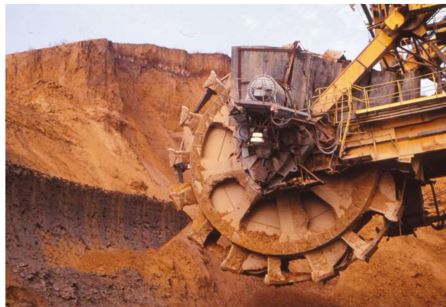
General view of the Chabařovice mine after the end of the mining activities, Retractable wheel excavator KU 300 mining a coal seam, author: Ing. Stanislav Štýs
